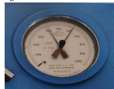
Figure 3.2 RCA COMPRESSIVE STRENGTH-640
